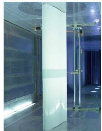
Wind tunnel tests to ensure highest aerodynamic efficiency of EUROS rotor blades
