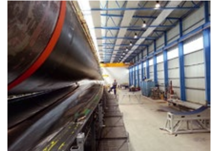
Offshore blade, length 80+ m, demoulding
