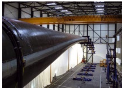
Offshore blade, length 80+ m, flapwise test
