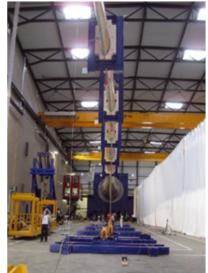
Offshore blade, length 80+ m, edgewise test
