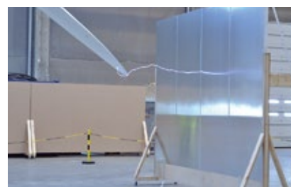
Lightning protection test, tip part
